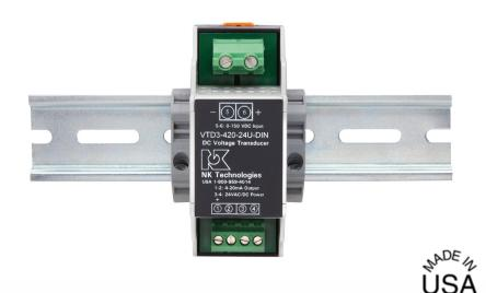
**VTD Series** Voltage Transducers are high-performance transducers for sensing voltage in DC powered installations. Applicable for use on circuits to 600 VDC, VTD voltage transducers provide a fully isolated, 4-20mA output proportional to rated nominal voltage in DC circuits. Housed in a slim, compact, easy-to-install DIN-rail mount enclosure, the VTD Series comes in a variety of nominal voltages.
